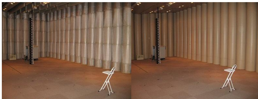
Figure 3 – Image of experimental environment (Left: Reverberation time 140 ms, Right: Reverberation time 1030 ms)
