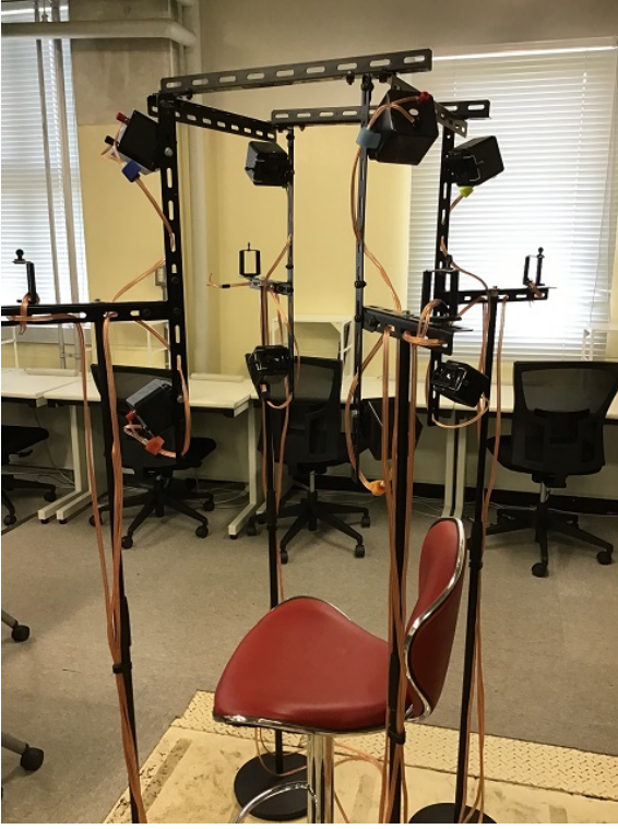
Fig. 12 Loudspeaker array in the localization test.
