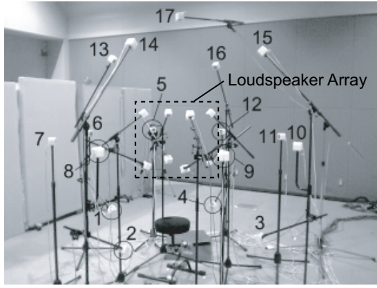
Figure 5: Setup of the loudspeaker array and loudspeakers for the control condition.
