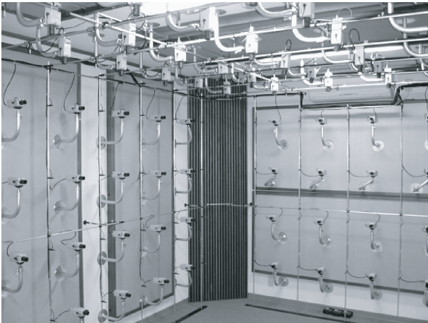
Fig. 6 Image of surrounding microphone array placed in the room [9].
