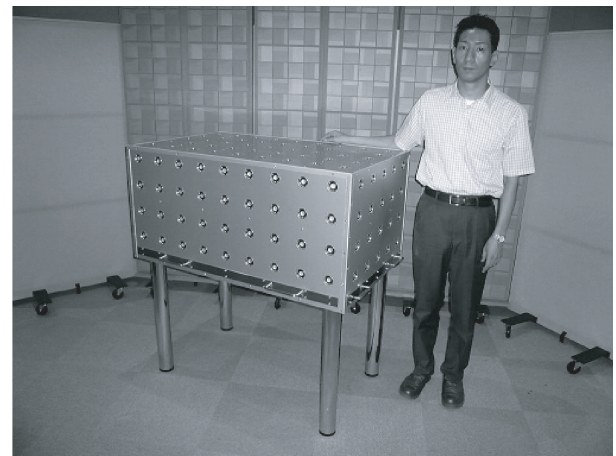
Fig. 8 Image of radiated loudspeaker array.
