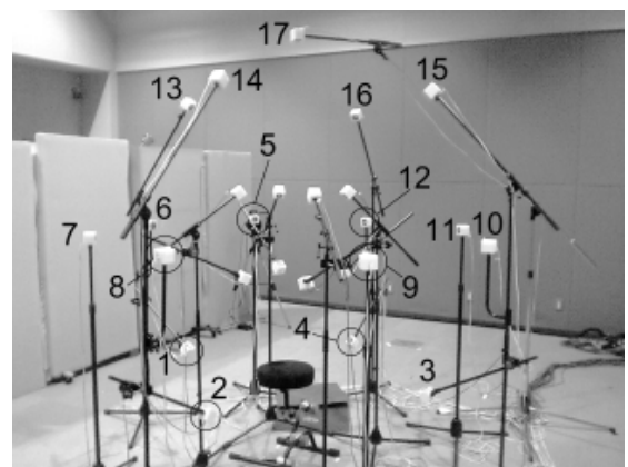
Fig. 4 Setup of the loudspeaker array and loudspeakers for control condition in the localization test
